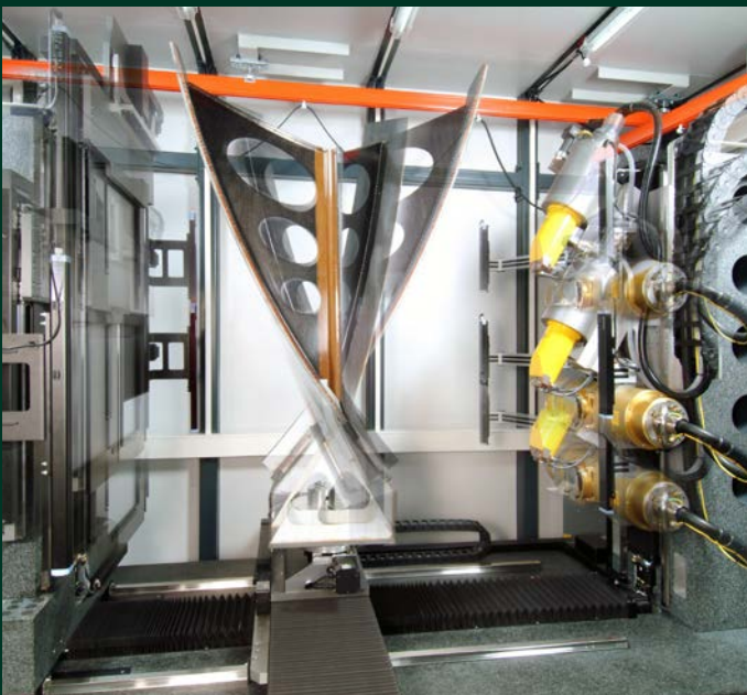
Phoenix V|tome|x L450: Movement of all axes for scanning a large crash spant. Courtesy of German Space Agency DLR.
